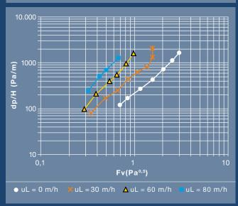
The new lattice-type random packing VFF-Gridlox is positioned almost plane during filling and enriches the VFF delivery program with a random packing of an inner structured pattern. The VFF-Gridlox is applicable in a wide range of applications and can be used as covering bed on top of the catalyst bed or as an entire random packing bed. The VFF-Gridlox is available in one dimension, the specific surface is approx. 290 m²/m³.
